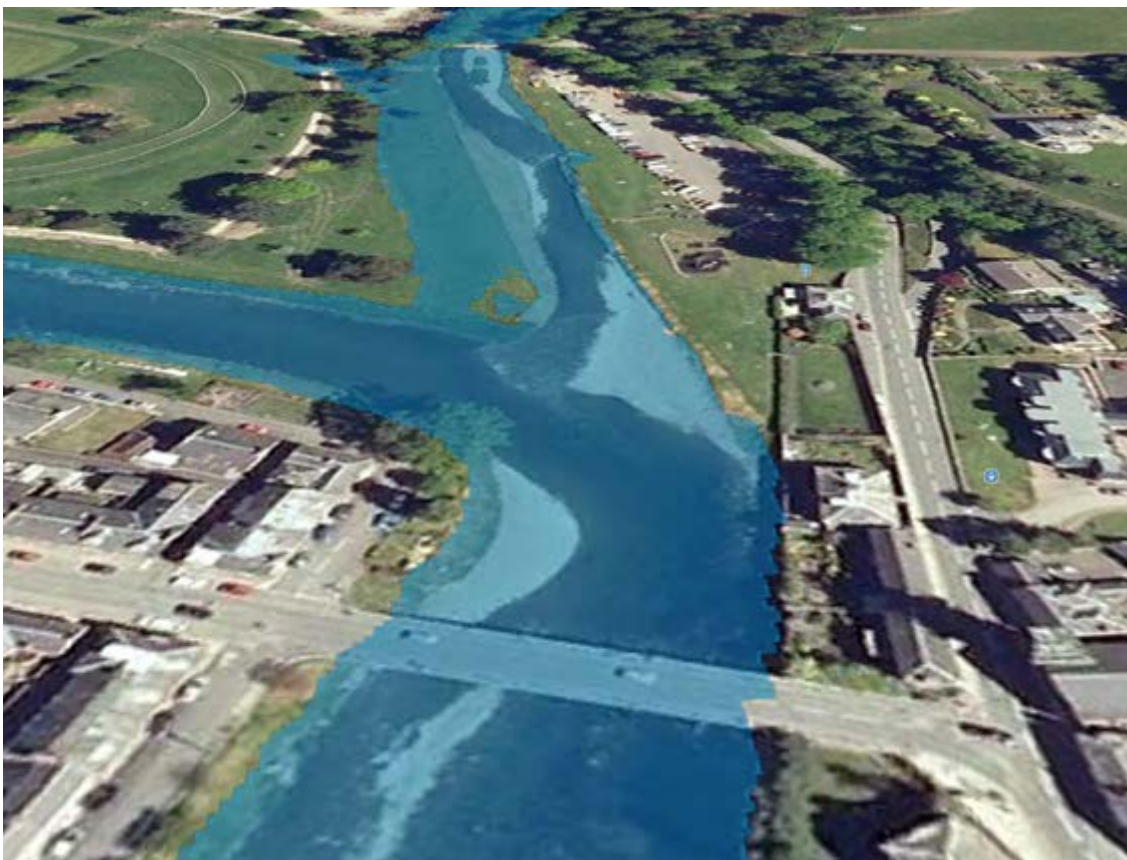
Model output at corresponding time superimposed onto Google Earth
