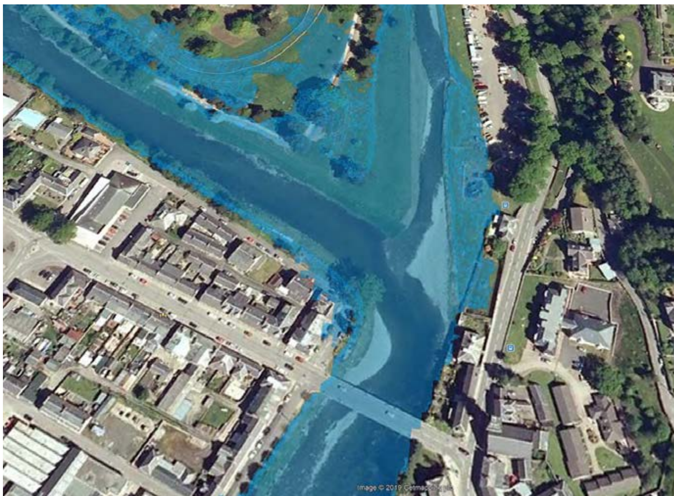
Model output at corresponding time superimposed onto Google Earth - Looking upstream from Thomas Telford Bridge
