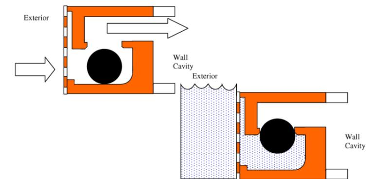
The Smart Airbrick is a straight replacement for a standard airbrick allowing free airflow under the floorboards eliminating the risk of damp and dry rot and stopping rodent infestation. During flood conditions 4 valve balls float on the floodwater automatically stopping the flow of water under the property.
