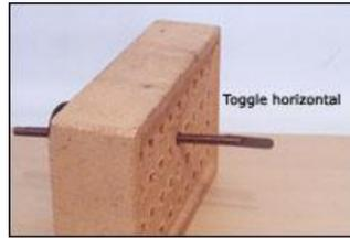
Insert rod through Ventguard and airbrick, turn rod vertical and tighten handle.
