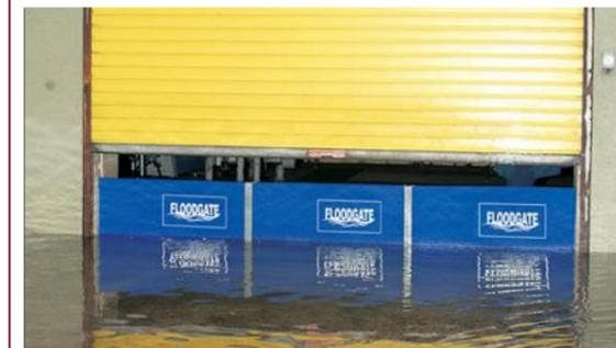
Floodgate comprises of a 25mm thick, steel boxed frame which expands telescopically on the horizontal and vertical plane. The steel frame is enveloped by a 7mm thick neoprene jacket which, when expanded, forms a waterproof seal between it and the aperture it is expanded into.
