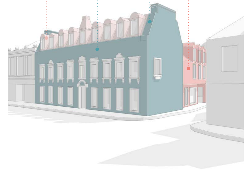
3D sketch from George Street showing proposed partial facade retention strategy combined with new build elements.
