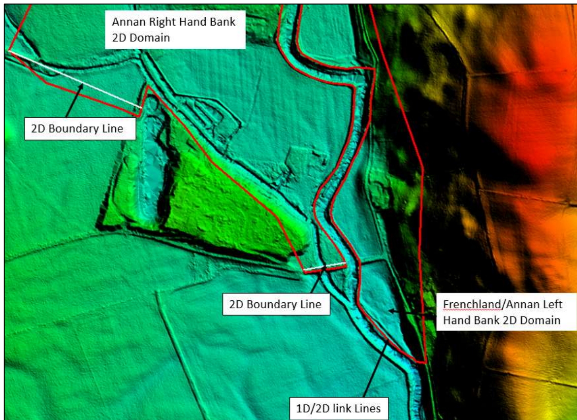
Figure 22: 2D downstream boundary
