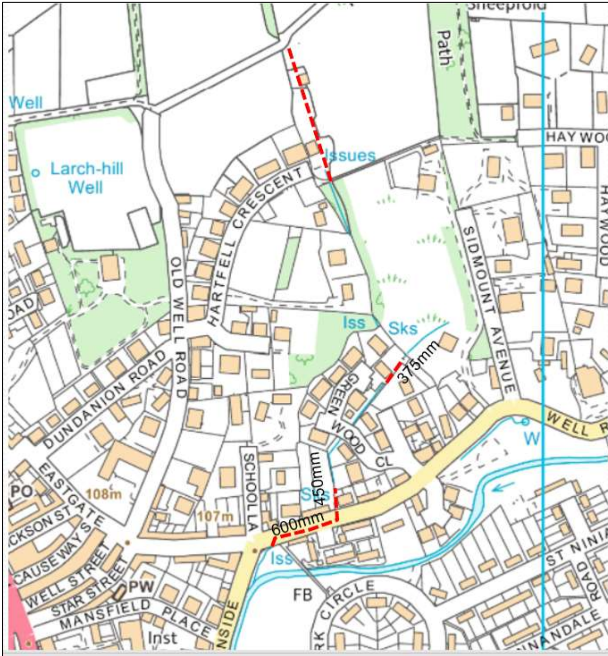
Figure 28: Indicative line of Greenwood Close culvert
