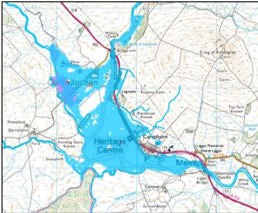
Figure 5: Approximate extent of SEPA 1 in 200 year fluvial flood maps of Carsphairn (reproduced manually by Kaya Consulting)
