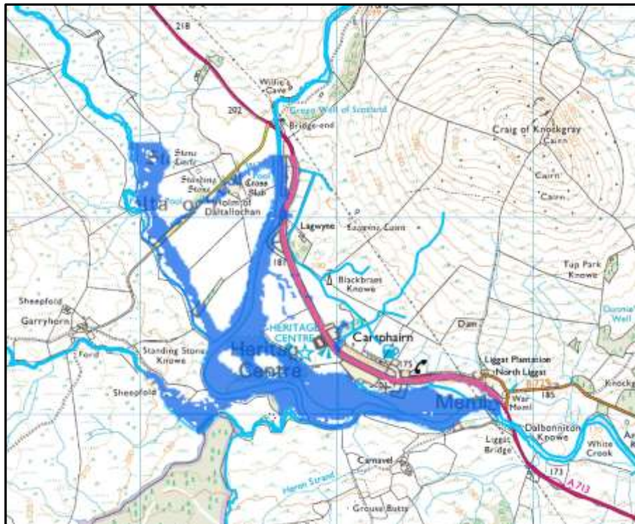
Figure 4: Approximate extent of SEPA 1 in 10 year fluvial flood maps of Carsphairn (reproduced manually by Kaya Consulting)
