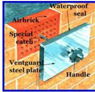
Insert rod through Ventguard and airbrick, turn rod vertical and tighten handle.
