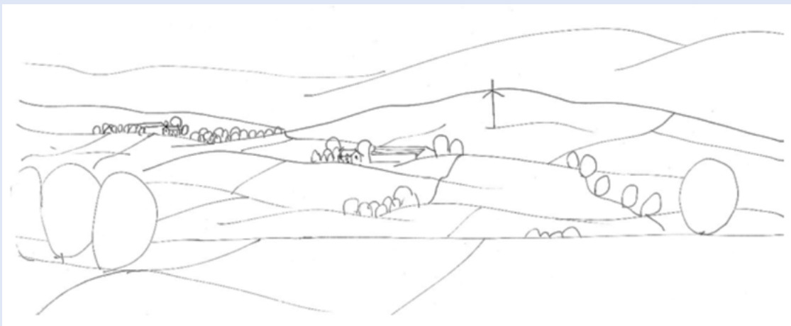
Landform shape and scale: Indicative 35m high turbine (4.5 x house height) located on the side of a hill, sited where there is a distinct fold in the landform. The turbine has been located on a hillside where there are no other features - like trees or houses - against which to gauge its height.
