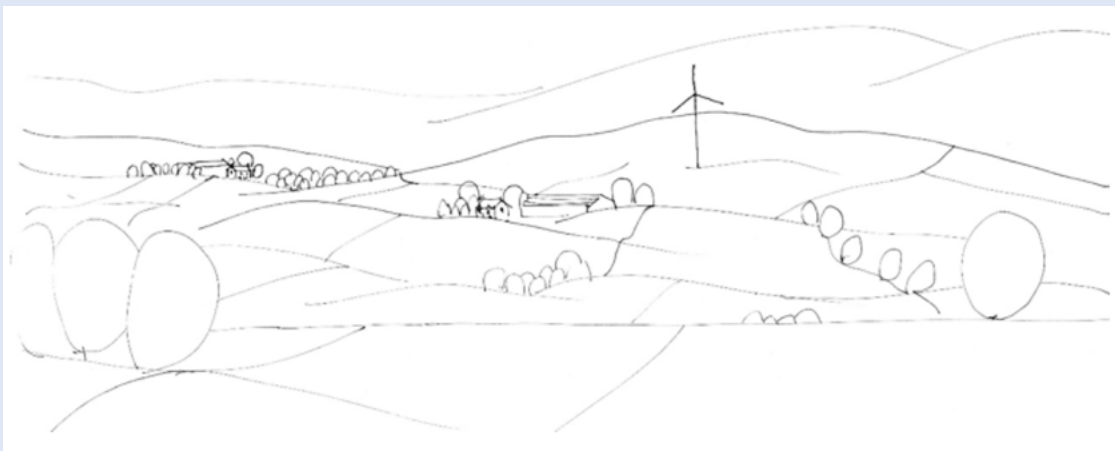
Landform shape and scale: Indicative 48m high turbine (6 x house height) located on the side of a hill, sited where there is a distinct fold in the landform. The taller the turbine, the more important it is that it is located where it is associated with landform scale, not the size of individual landscape features - this size would be more readily accommodated further away from the farm.
